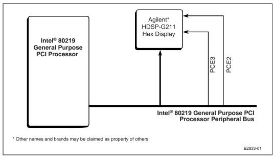
Redboot\* uses address range  $0xFE84\ 0000$  -  $0xFE84\ 0FFF$  for the left 7-segment LED (PCE3) and address range  $0xFE85\ 0000$  -  $0xFE85\ 0FFF$  for the right 7-segment LED (PCE2).
